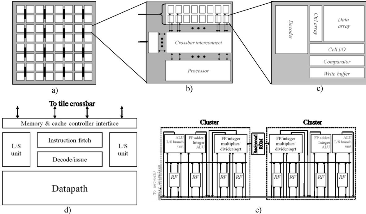
**Figure 1. Smart Memories Architecture: a) chip floorplan; b) tile block diagram; c) reconfigurable memory block diagram; d) reconfigurable processor; e) shared processor data-path**
