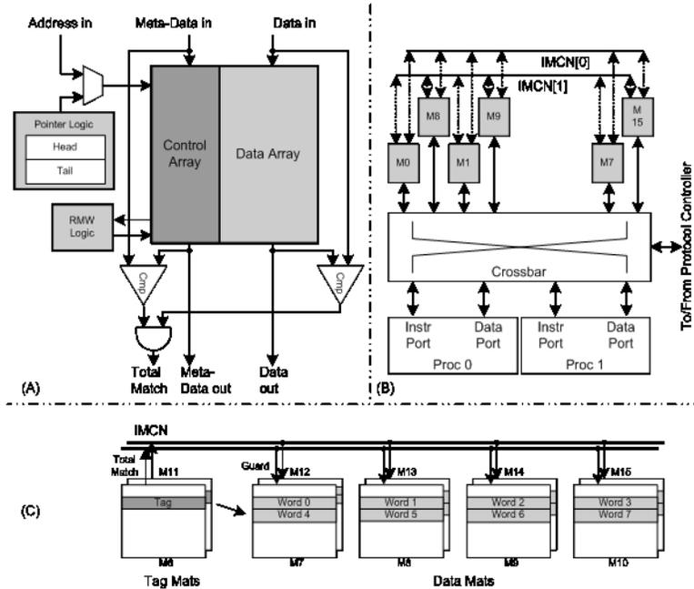
**Figure 3. Tile memory organization: a) block diagram of the memory mat; b) tile crossbar and IMCN; c) example cache configuration**
