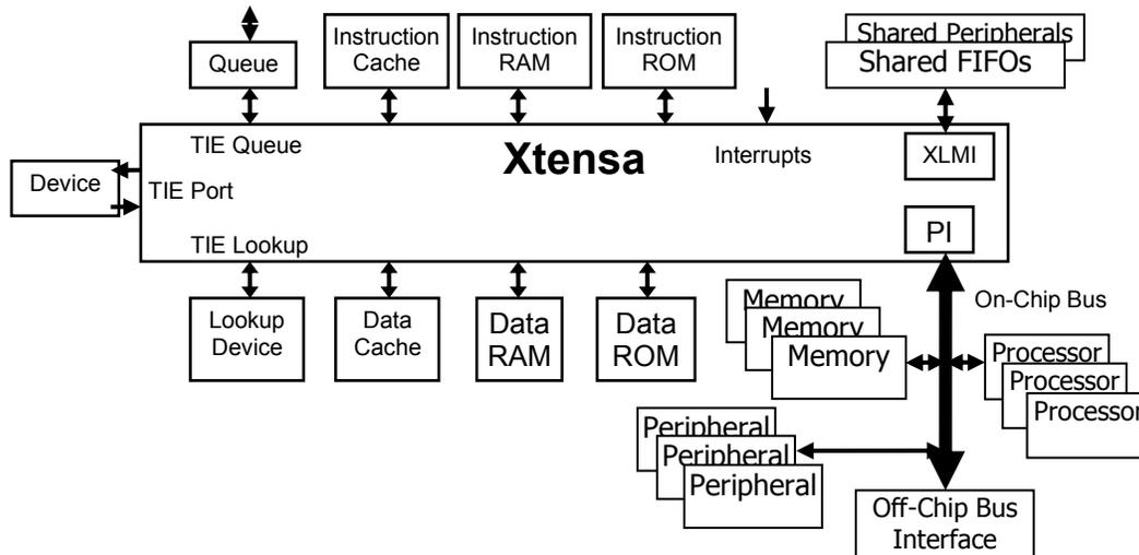
**Figure 2. Tensilica Processor Interfaces**
