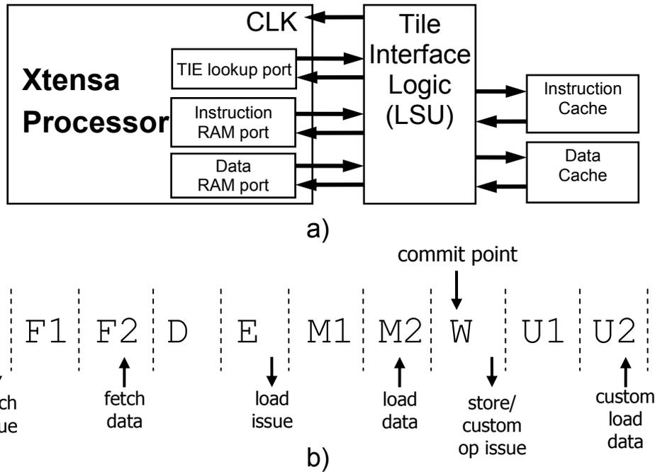
**Figure 4. a) Interfacing Tensilica processor to Smart Memories; b) processor pipeline**
