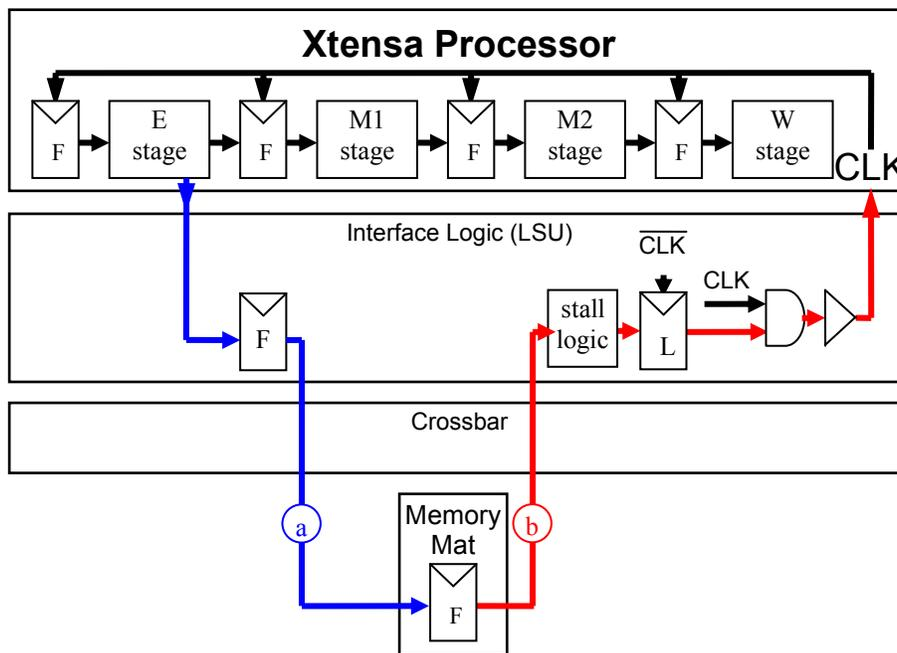
Figure 6. Tile timing critical paths: a) forward path from processor to local memory/cache; b) reverse path from local memory/cache to processor
