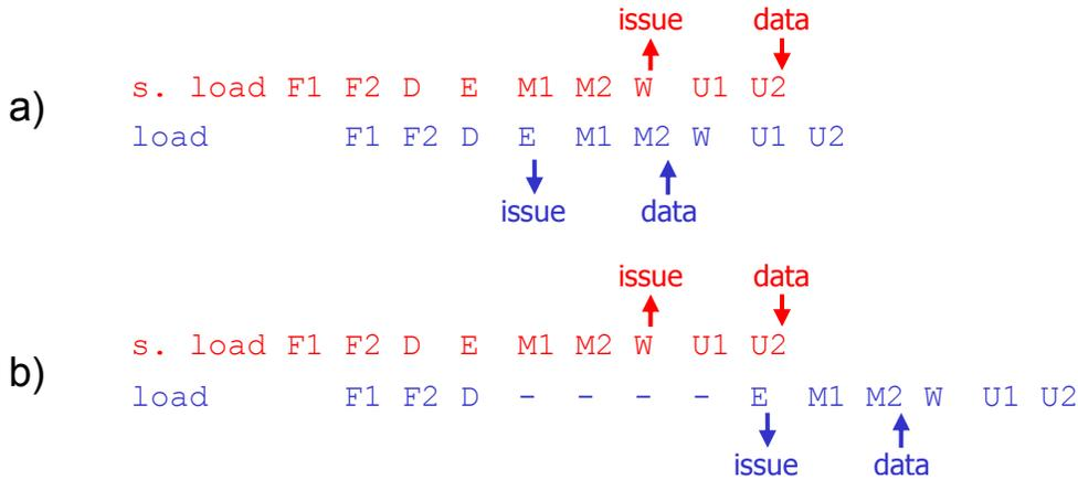
Figure 5. Ordering of memory operations: a) without interlock, b) with interlock
